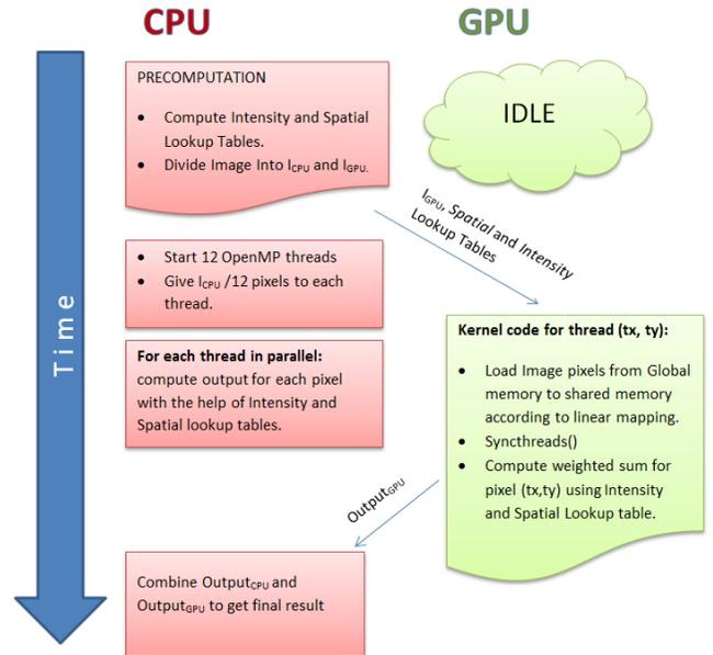
Fig. 4. flow of the hybrid algorithm with time
